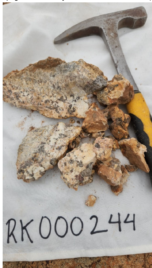
Figure 12: Pegmatitic lens from location RK0000244 (12ppm Li and 81ppm Ta).
