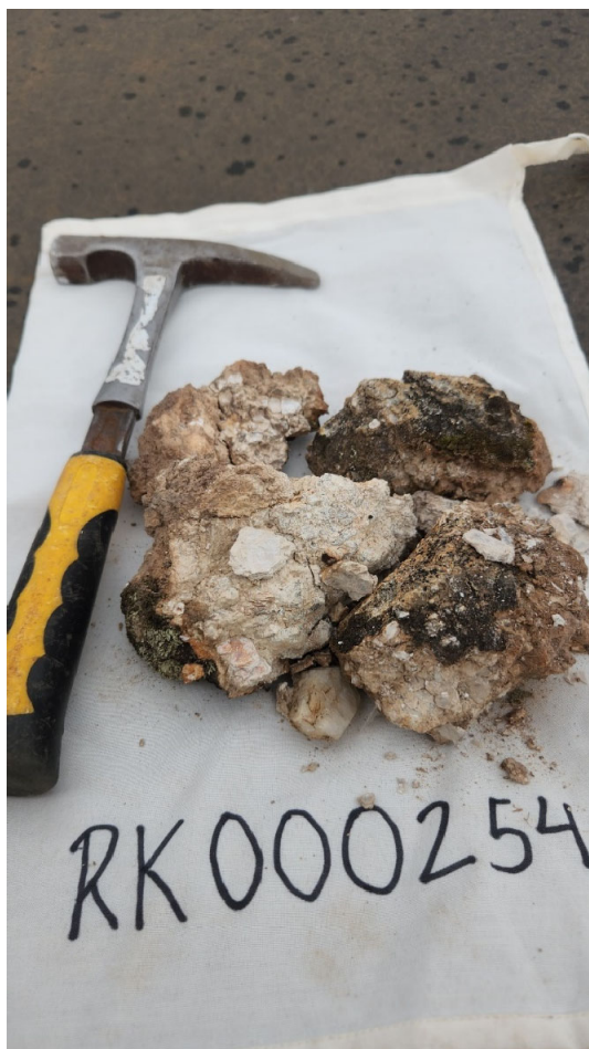
Figure 13: Weathered pegmatitic vein from location RK0000254 (54ppm Li and 48ppm Ta).
