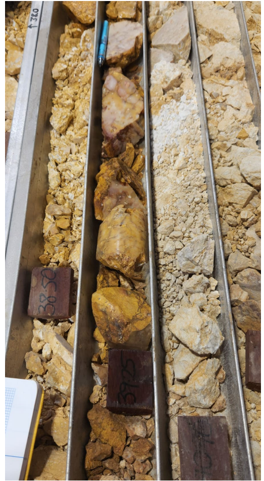
Figure 3: DDB-20 diamond drill core with zones of interest for full suite analysis, previous intersection of 1m at 51g/t gold from 39m. (left image is a zoomed in version of right).
