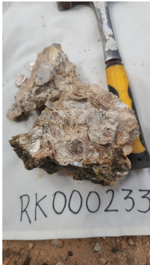
Figure 11: Coarse grained pegmatitic rocks from location RK0000233 (94ppm Li and 22ppm Ta).
