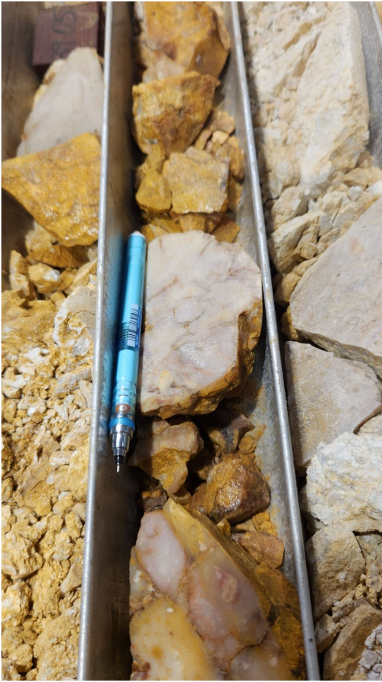
Figure 3: DDB-20 diamond drill core with zones of interest for full suite analysis, previous intersection of 1m at 51g/t gold from 39m. (left image is a zoomed in version of right).
