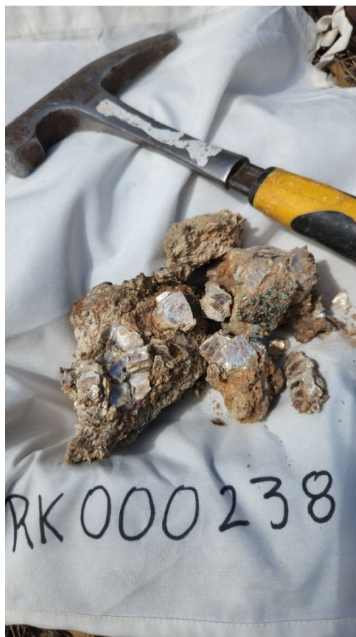
Figure 9: Coarse grained pegmatitic rocks from location RK0000238 (165ppm Li and 38 ppm Ta).
