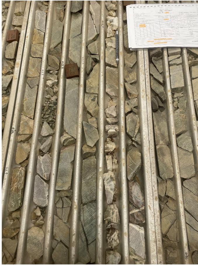
Figure 2: Drillhole DDB-1 diamond core tray, zone of pegmatite interest from 73-74m for full suite analysis.
