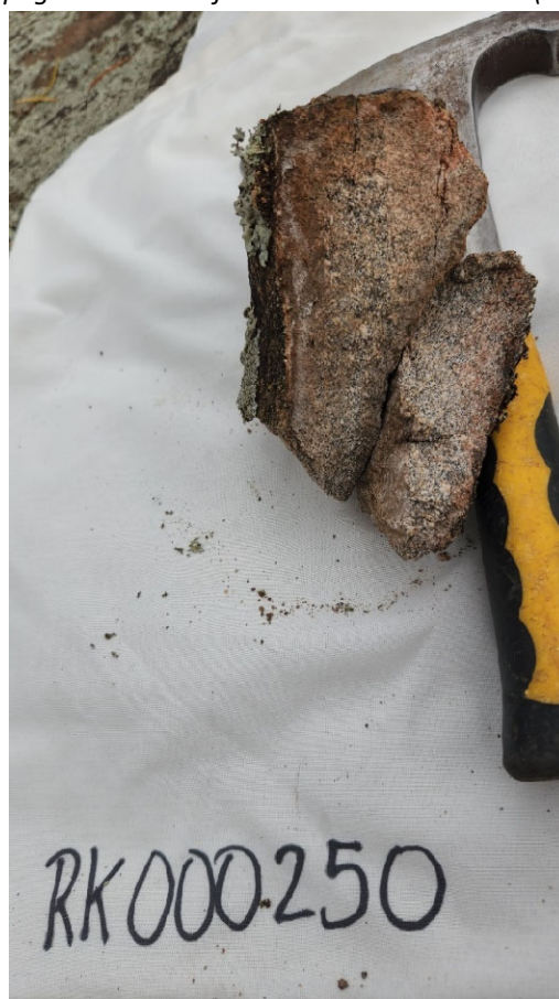
Figure 10: Contact with coarse grained pegmatitic vein from location RK0000250 (128 ppm Li).
