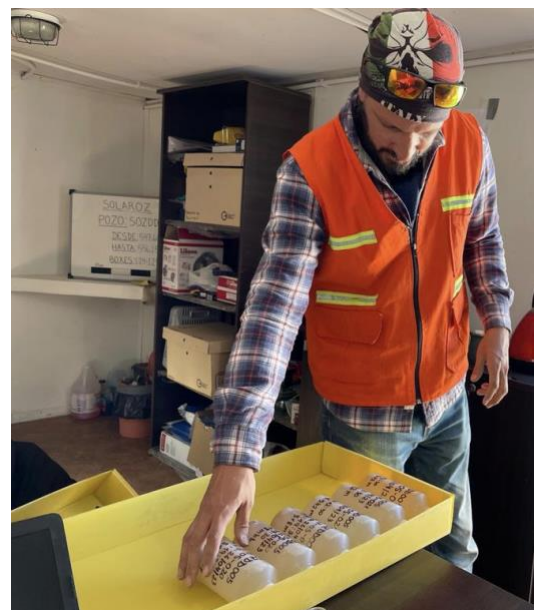
Figure 5: Collection of Brine Samples for Assaying
