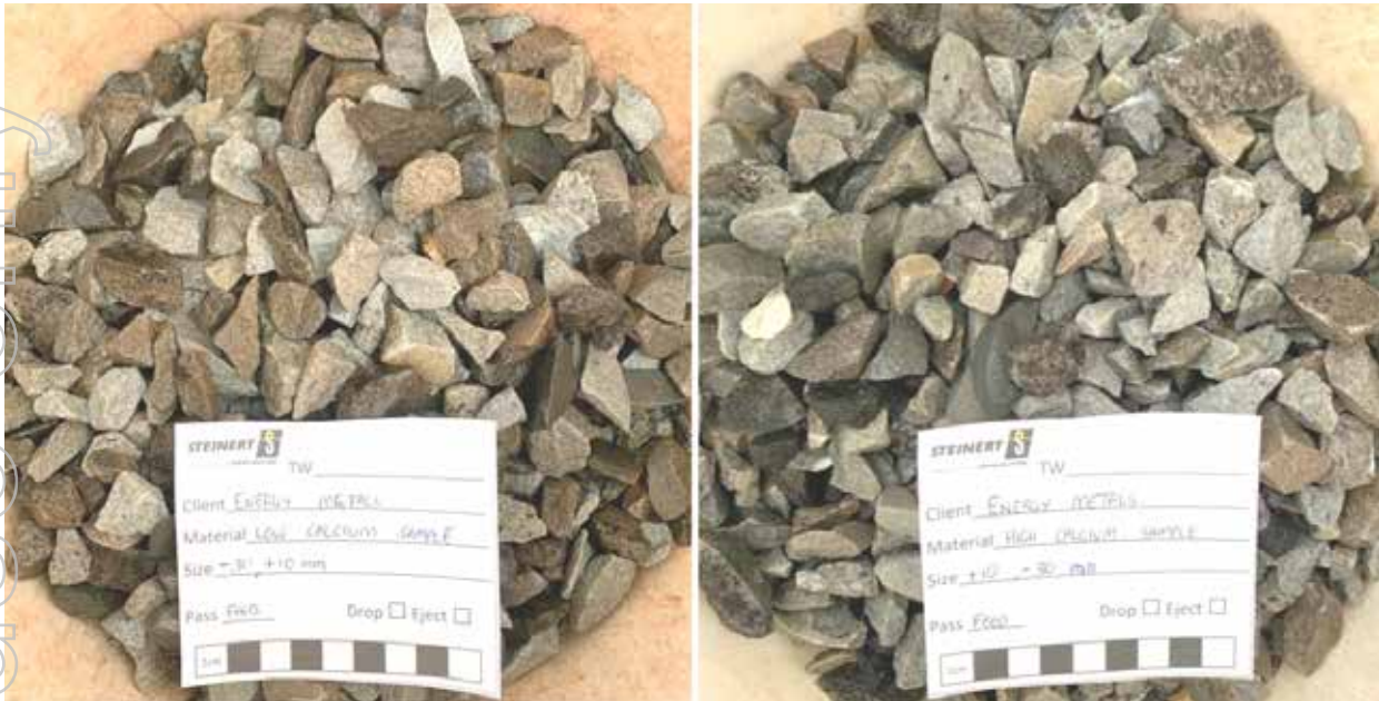
Figure 5 – Low-carbonate (left) and high-carbonate (right), +10mm feed samples for ore sorting.
