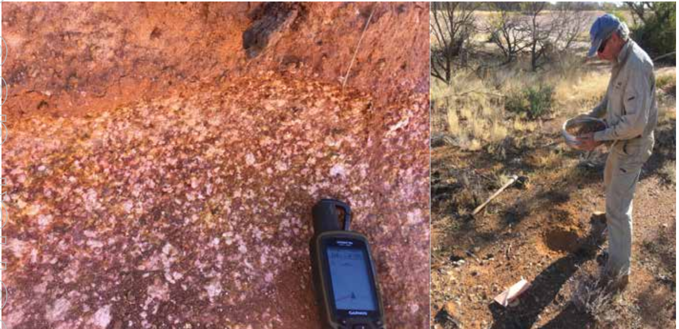
Figure 7 – Clay zone overlying granitic saprolite (left) and soil sampling (right) at the Crystal Creek prospect.
