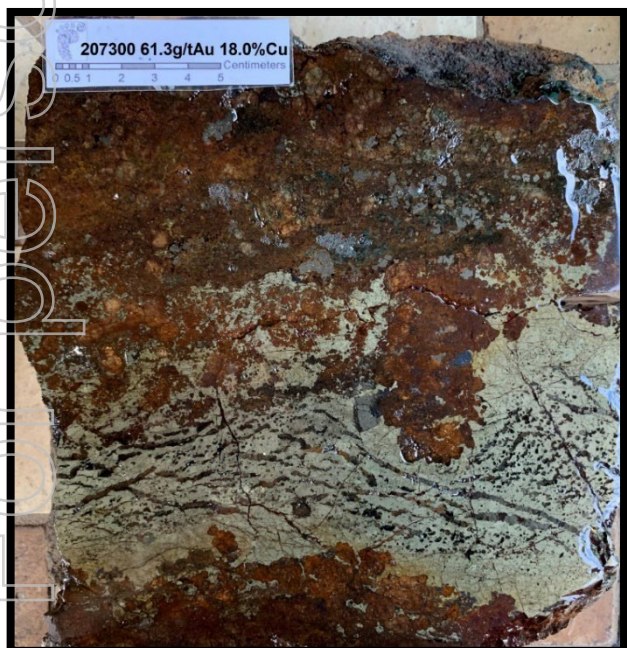
Photo 1c High grade chalcopyrite-garnet-magnetite polished rock sample from Leah's Lode outcrop, 2m from trench - 61.3g/t Au, 18% Cu, 135g/t Ag 2 .
