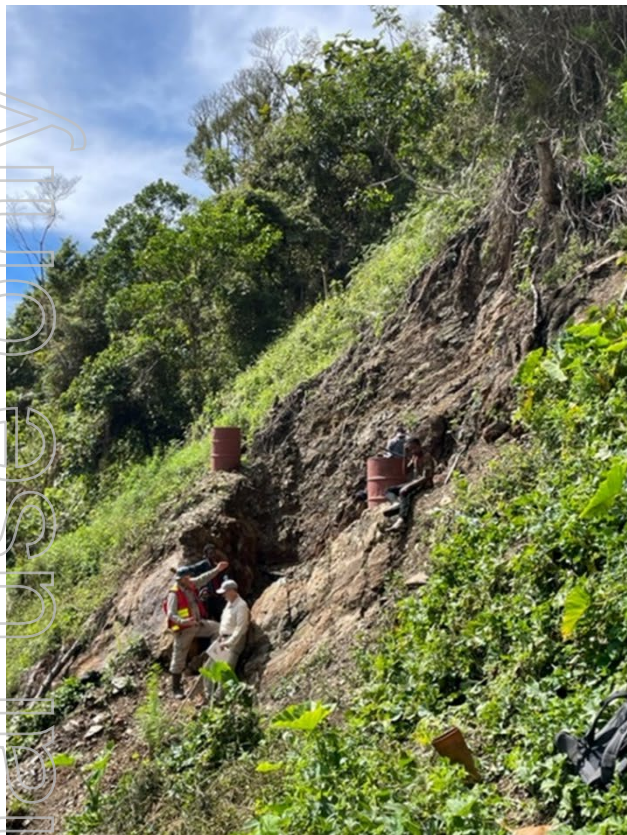
Photos 1a & b Photo 1a: Leah's Lode is a 2022 discovery. Trenching (FPRTR4) has delivered 8m @ 11.5g/t Au, 2.6% Cu, 24g/t Ag 2 . Photo 1b: Clearly visible copper oxide mineralisation exposed within the trench.
