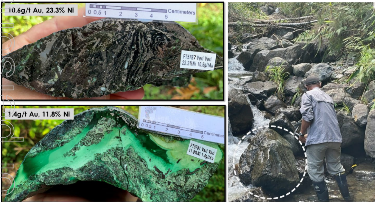
Photo 2: Veri Veri creek float samples include massive nickel sulphide minerals (heazlewoodite, millerite, pentlandite) and nickel-bearing silicates including serpentinite and garnierite. Photo Right: boulder with nickel sulphides in creek.
