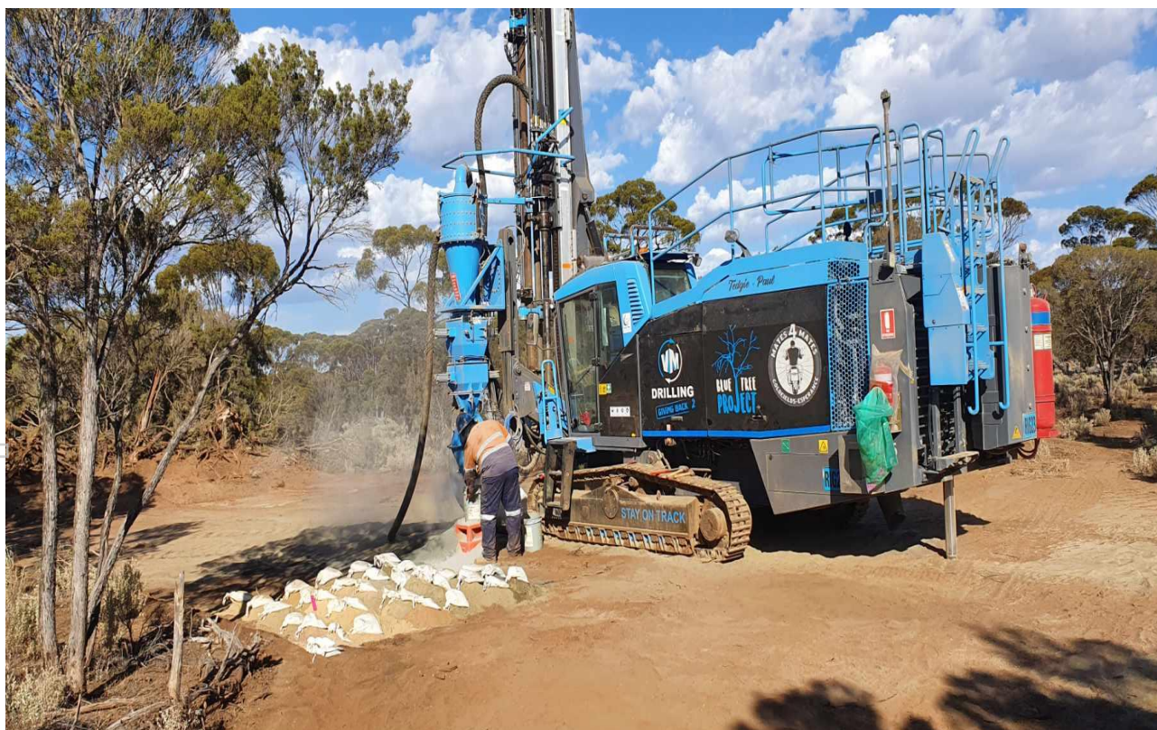
Grade control drilling: Jeffreys Find.
