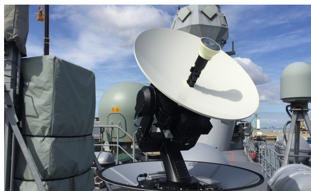
"Cobra" Maritime SATCOM Terminal Installation with the RAN
