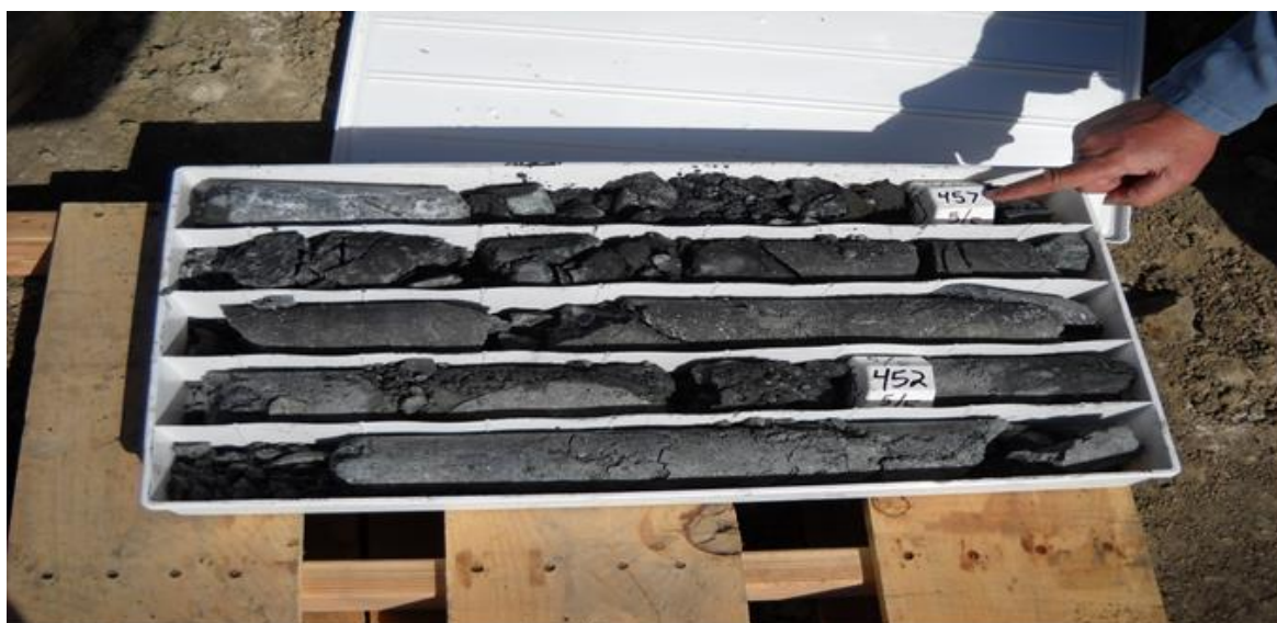
Figure 6: Drill cores showing metasomatic magnetite
