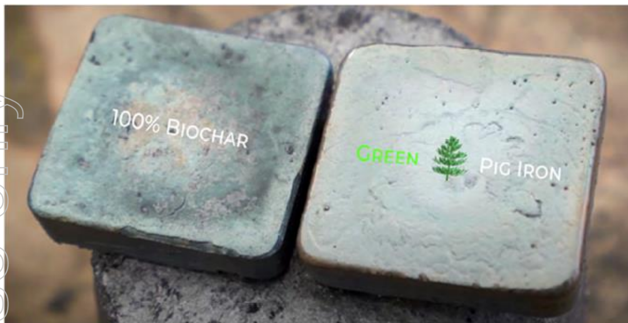
Figure 3: Biochar Green Pig Iron
