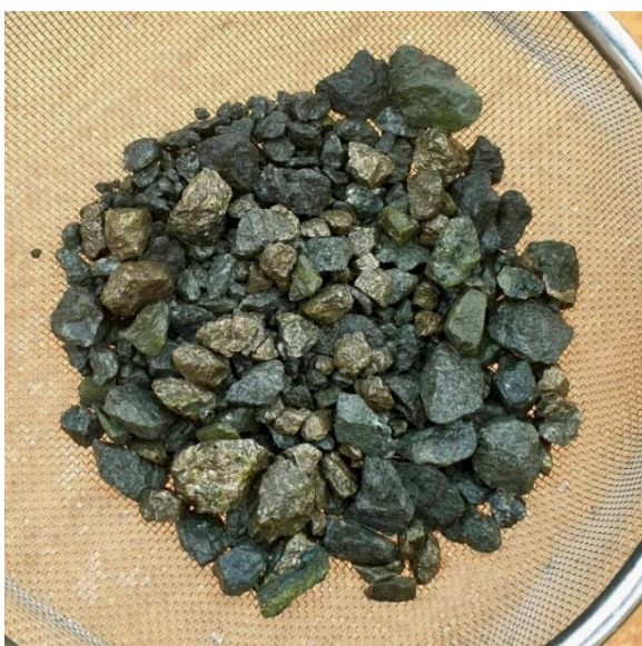
Figure 1: RC chips from REYRC002 80-81m comprised of pyrrhotite, pentlandite and chalcopyrite within the Money Intrusion. This interval was drilled in 2022 and returned 0.85% Ni, 0.77% Cu, 0.46% Co and 0.17g/t 3PGE. REYRC002 was targeting a ~180S conductive plate.
