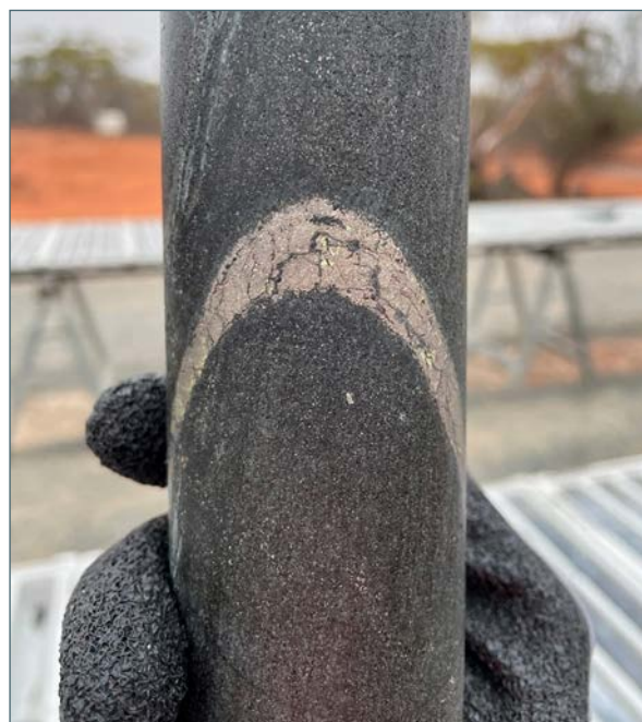
Photo 3: Cross-cutting massive sulphide vein from RKDD082W1 from 819.3m, NQ2
