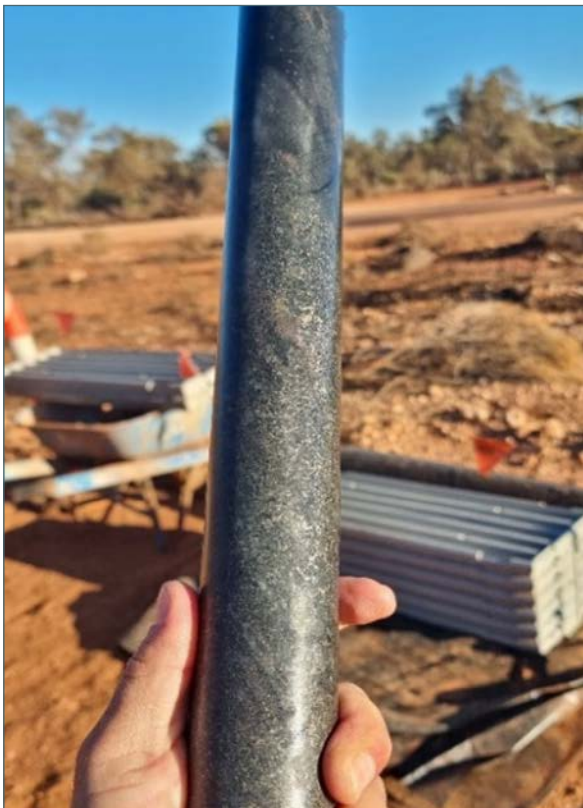
Photo 2: Heavy disseminated sulphide intrusion from RKDD081 from 840m, NQ2
