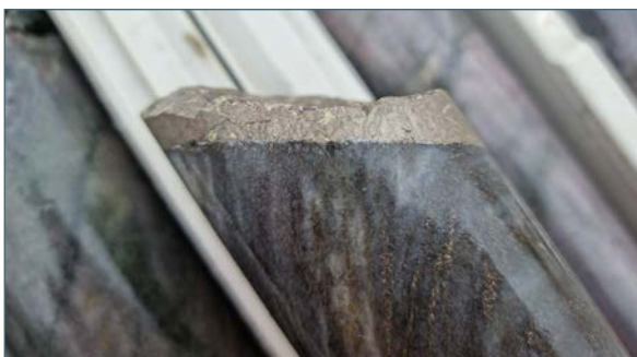
Photo 4: Cross-cutting massive sulphide vein from RKDD083 from 480m, NQ2
