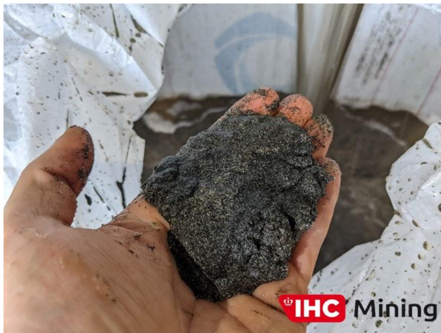
Plate 5 – Washed sand ready for industrial sand and magnetite-heavy mineral recovery ( +2\text{mm} -45\mu\text{m} )
