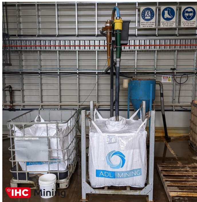
Plate 4 – Slimes removal (material <45\mu\text{m} )
