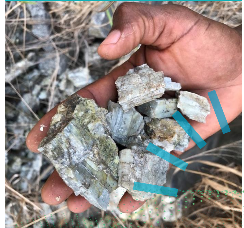
Coarse spodumene concentrate
