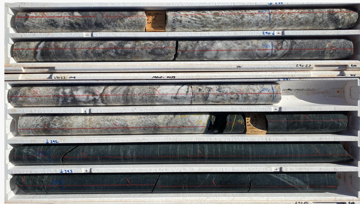
Manna core; white spodumene mineral and two waste rock types, a coarse grain dark grey magnetic mafic and a fine grain dark grey/green basalt
