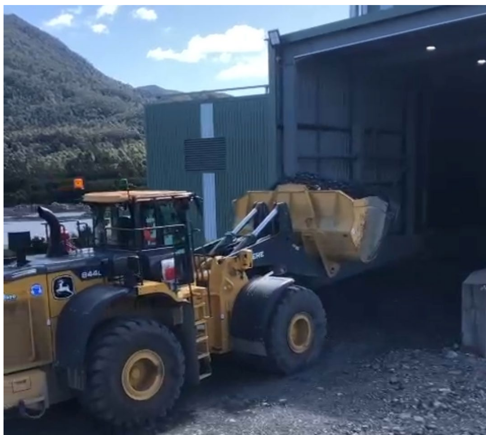
Figure 2. Loader feeding ore from the run-of-mine pad to the crusher.
