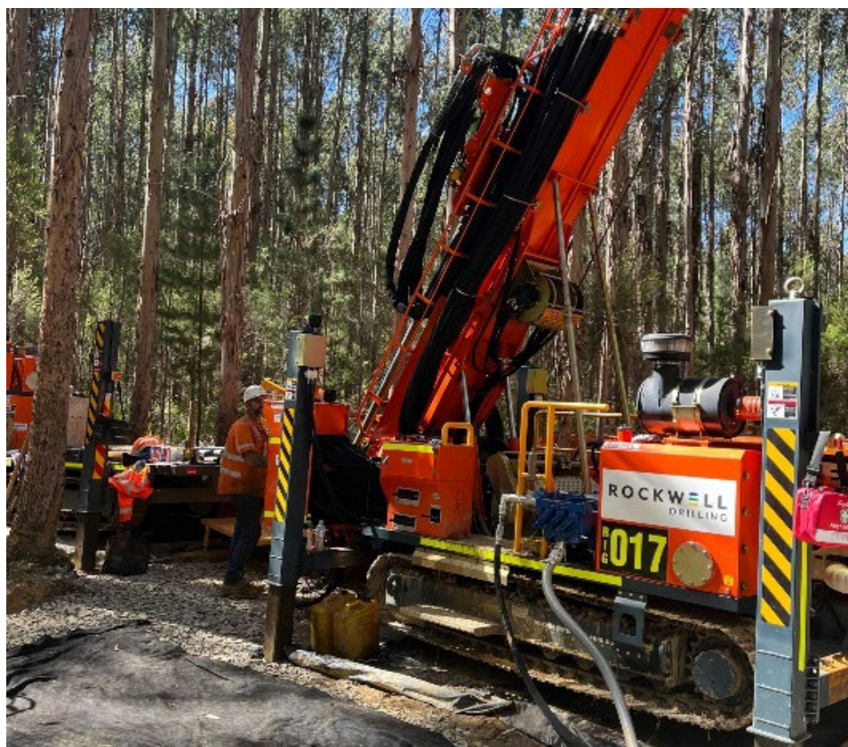
Figure 5. Exploration Diamond Drill at Melba.
