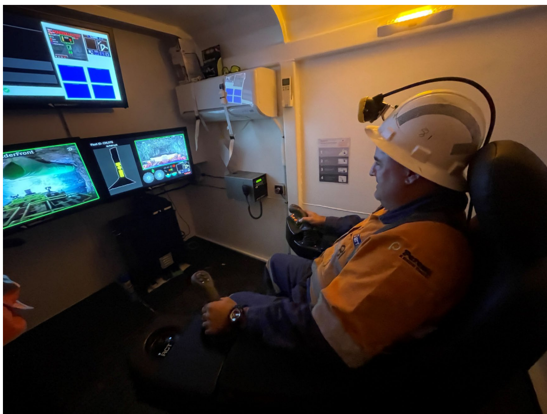
Figure 3. Remote bogging from portable operator station.
