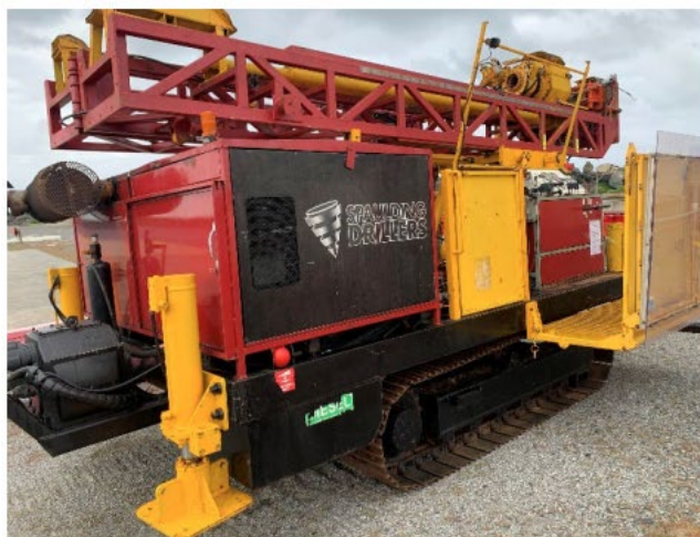
Figure 11 - Core Drill Rig at Dolphin Tungsten Mine
