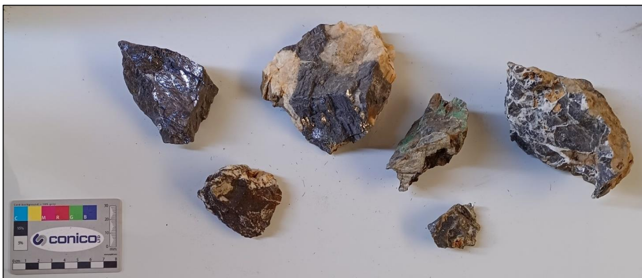
Figure 9. Nuldal rock chip sample 9968. Quartz vein-hosted massive galena with malachite staining, containing 83 g/t Ag, 22.2% Pb and 0.2% Zn.
