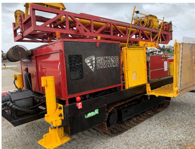
Figure 3 - Core Drill Rig at Dolphin Tungsten Mine
