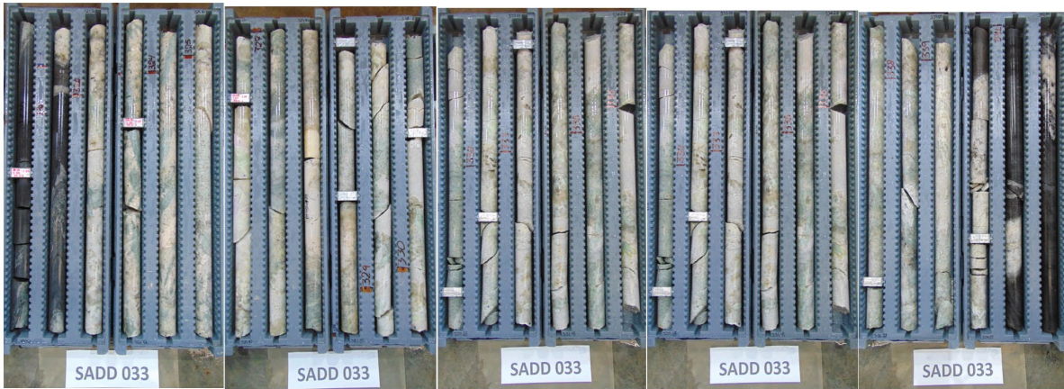
Figure 2: Colina West drill hole SADD033 – pegmatite intersection 319.40m – 341.94m (18.71m @ 1.32% \text{Li}_2\text{O}^2 )
