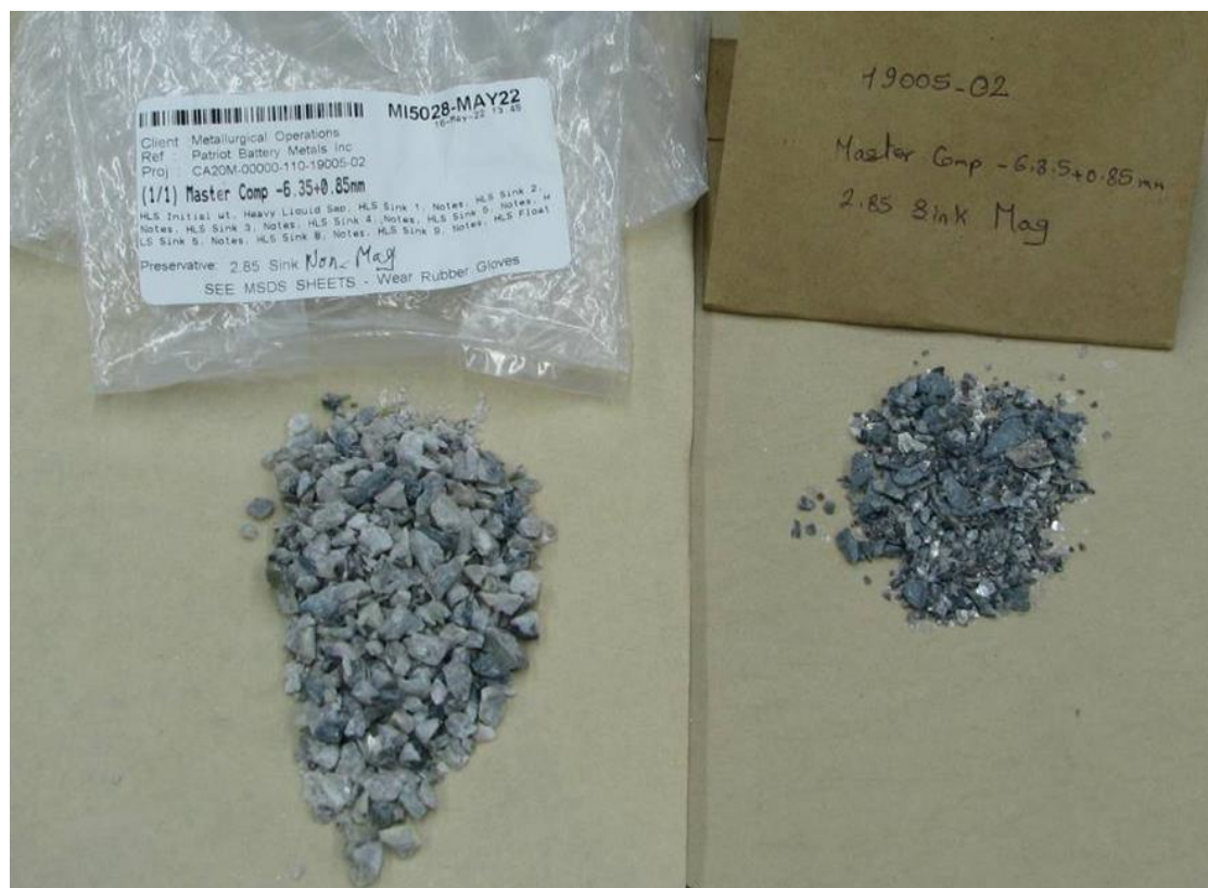
Figure 12: Non-magnetic (left) and magnetic (right) products on HLS sink (2.85 SG) following -6.3 mm crush. Non-magnetic concentrate grades 6.23% \text{Li}_2\text{O} and 0.66% \text{Fe}_2\text{O}_3
