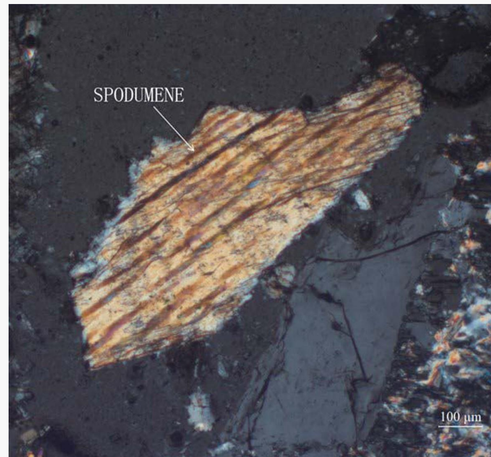
Electron microscope image of a lithium bearing spodumene monocrystal from the Marble Bar metallurgical test work.
