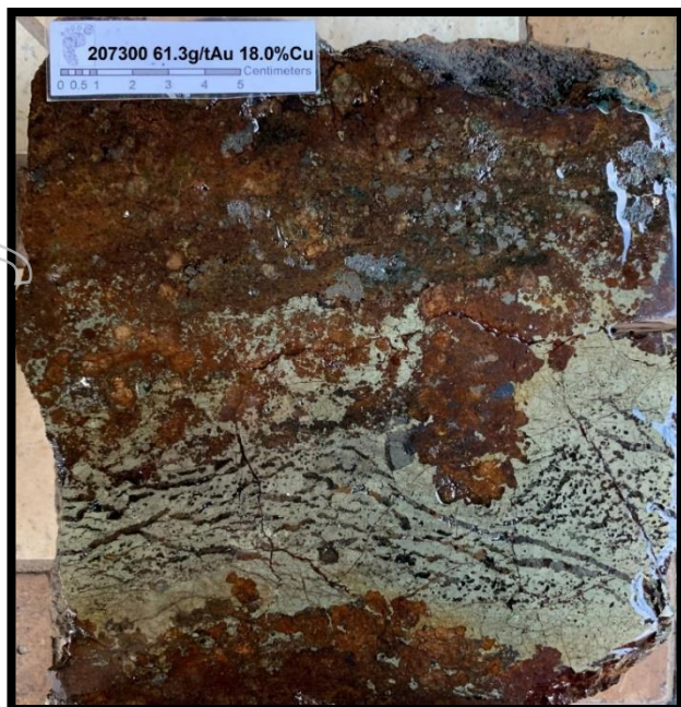
Photos 1a, b & c. Photo 1a: Leah's Lode is a 2022 discovery. Trenching (FPRTR4) has delivered 8m @ 11.5g/t Au, 2.6% Cu, 24g/t Ag. Photo 1b: Clearly visible copper oxides exposed within the trench. Photo 1c: High grade chalcopyrite-garnet-magnetite polished rock sample from Leah's Lode outcrop, 2m from trench - 61.3g/t Au, 18% Cu, 135g/t Ag (Table 3).
