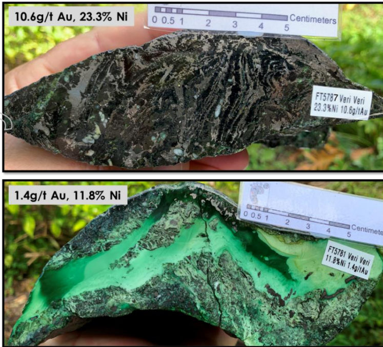
Photo 2: Veri Veri creek float samples include massive nickel sulphide minerals (heazlewoodite, millerite, pentlandite) and nickel-bearing silicates including serpentinite and garnierite. Photo Right: boulder with nickel sulphides in creek. Samples taken by Footprint, see Table 4 and JORC tables in this announcement.
