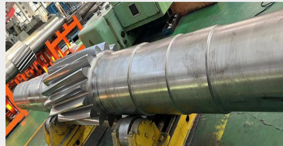
The teeth cutting stage for pinion finished
