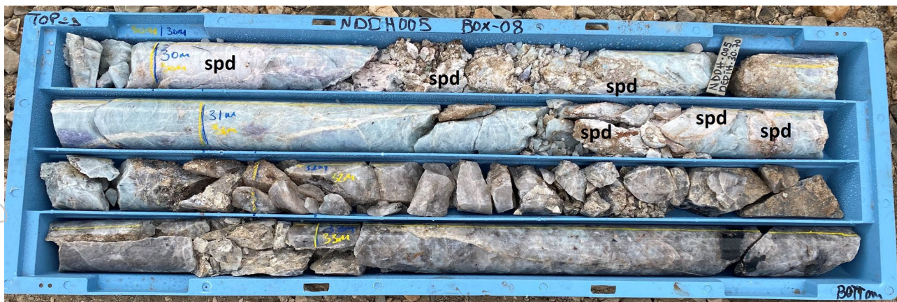
Figure 14: NDDH005 Core-tray #8. Spodumene labelled spd. Pale blue = albite (variety cleavelandite), purple = lepidolite, grey = quartz
