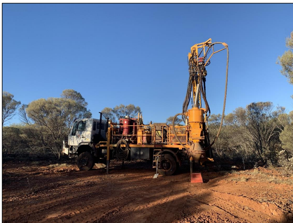
Figure 1 - RC drill rig set up at Weelarrana Manganese Project
