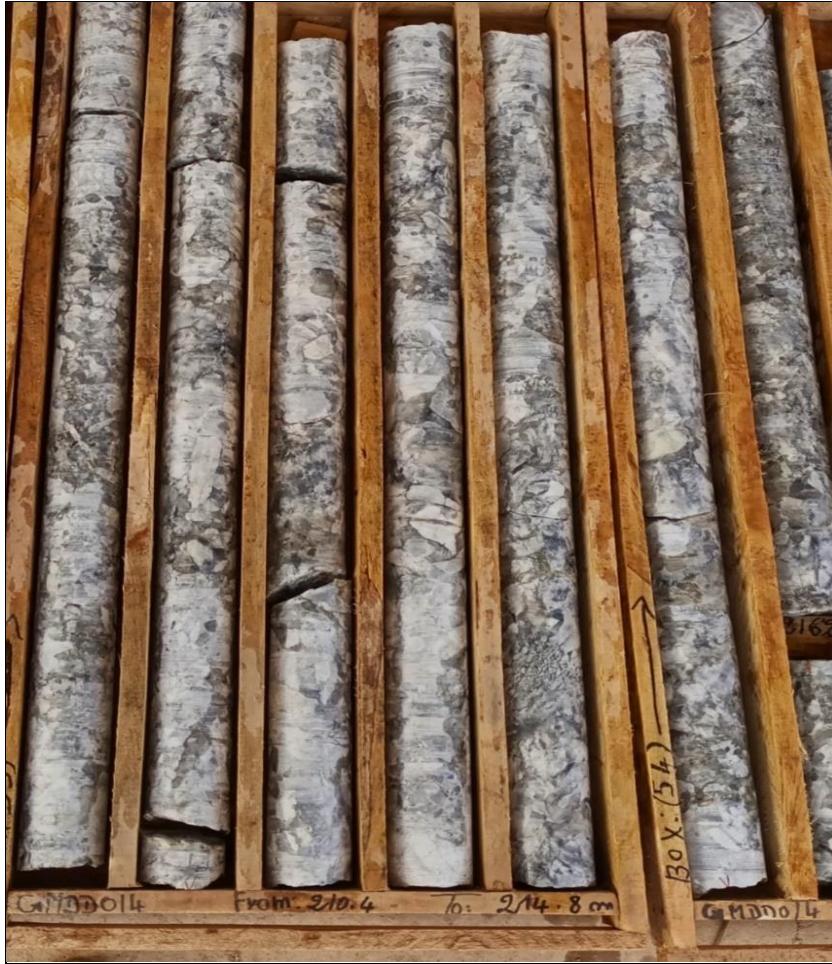
Figure 2 Typical coarse grained spodumene pegmatite from GMDD014 (210.4 m - 217 m)
