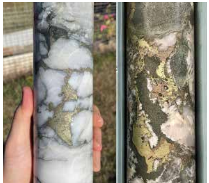
BTDD005 – 699.9m (left), 708.5m (right) – buck quartz vein with chalcopyrite-pyrite-pyrrotite infill.
