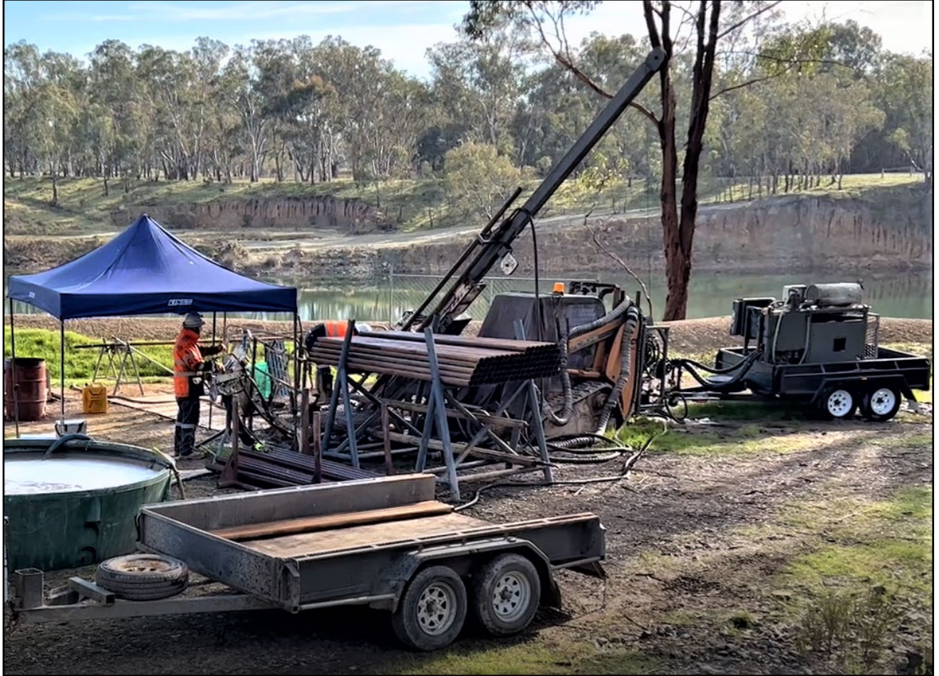
Photo 1 Contract diamond drilling rig positioned on the south side of the West Pit at the Nagambie Mine
