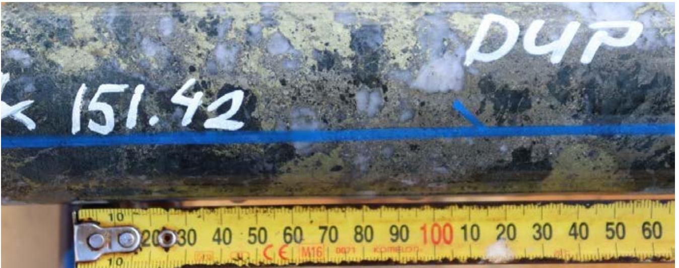
HMTRDD001 151.5m Chalcopyrite-Pyrrhotite as matrix infill in a quartz vein breccia. Main Trafalgar lode. The interval 151.42-152.55 assayed 0.5g/t Au and 7.65% Cu.
