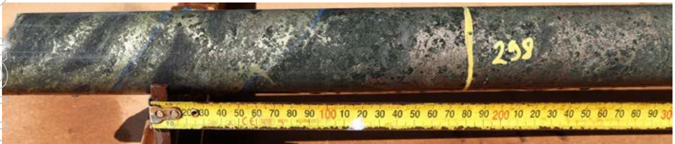
HMLVDD001 at 258m down-hole. Example of chalcopyrite-pyrrhotite mineralisation encountered in the hangingwall sulphide zone at Ajax east (ASX Announcement 29 June 2022).
