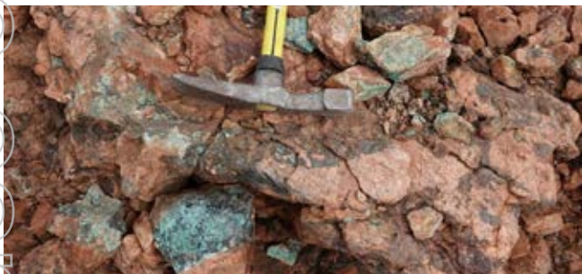
Breccia with coarse albite actinolite magnetite infill and abundant malachite on fractures.
