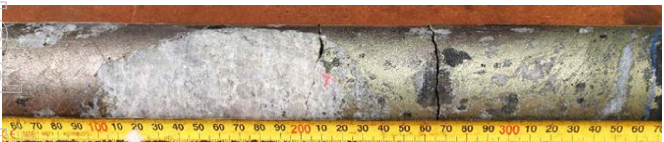
HMLVDD001 at 342.7m down-hole. Example of chalcopyrite-pyrrhotite mineralisation encountered in the footwall sulphide zone at Ajax east (ASX Announcement 29 June 2022).
