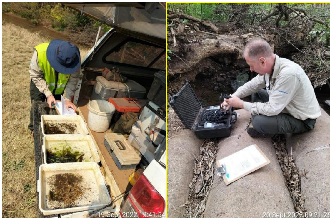
Figure 7,8: Samples taken to determine the assessment of the habitat integrity of the river. Surface water quality variables measured a Hach HQ40d Multimeter
