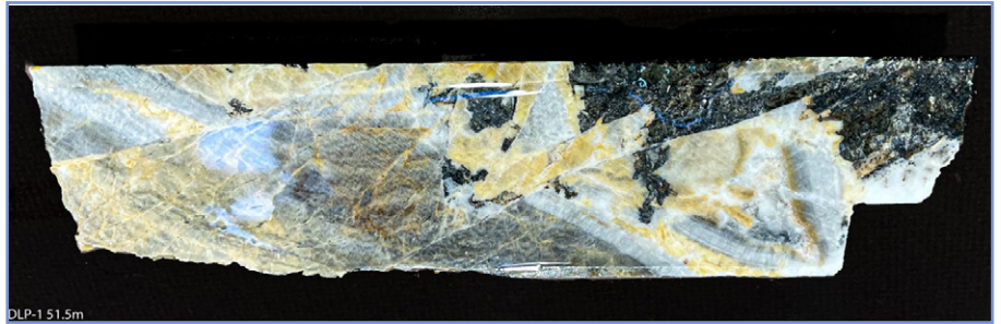
Figure 5 Example of coarse sphalerite infill (black) in BHP's diamond hole DLP-1 (51.5m depth).
