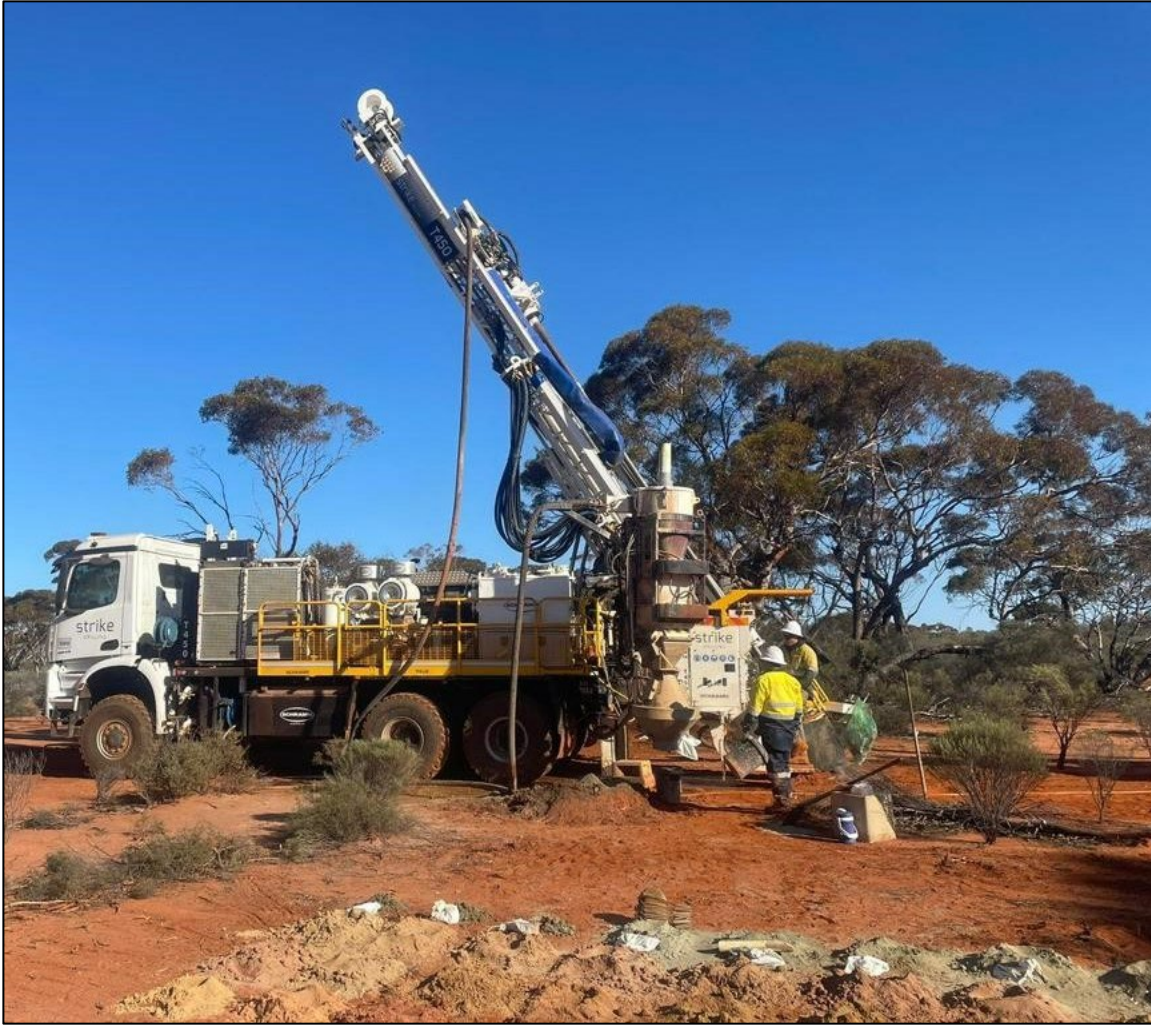
Figure 9. AC drilling at Emu Lake – September 2021
