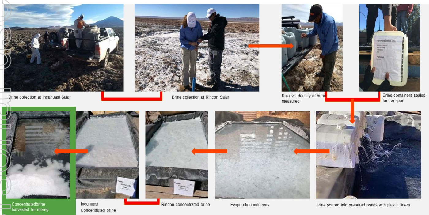
Figure 4: The brine blending process
