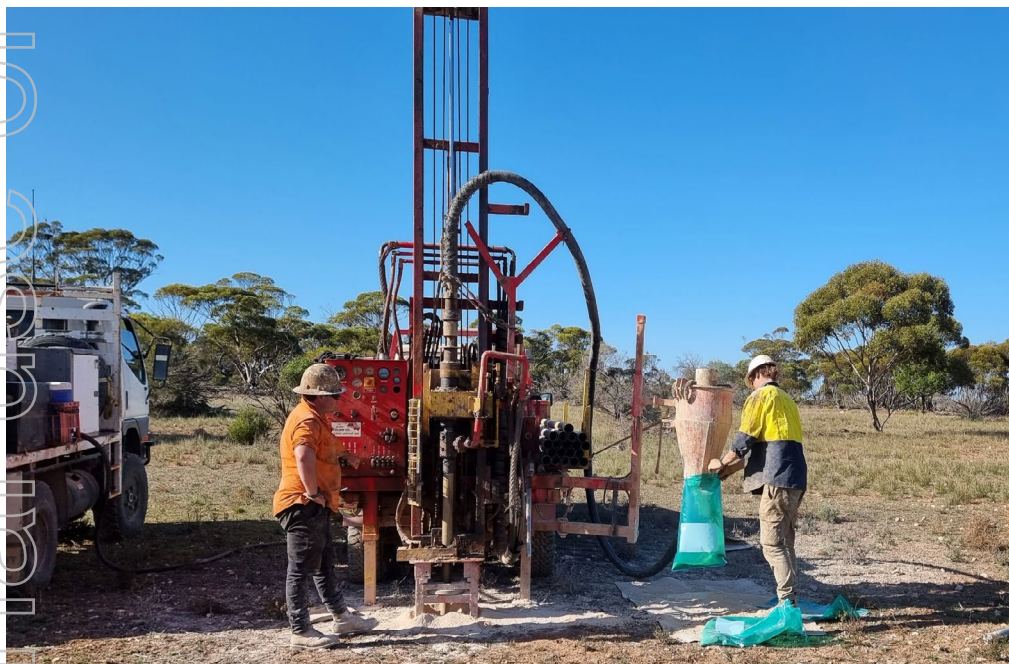
Figure 6: Drilling at the Eyre Peninsula Kaolin-Halloysite Project
