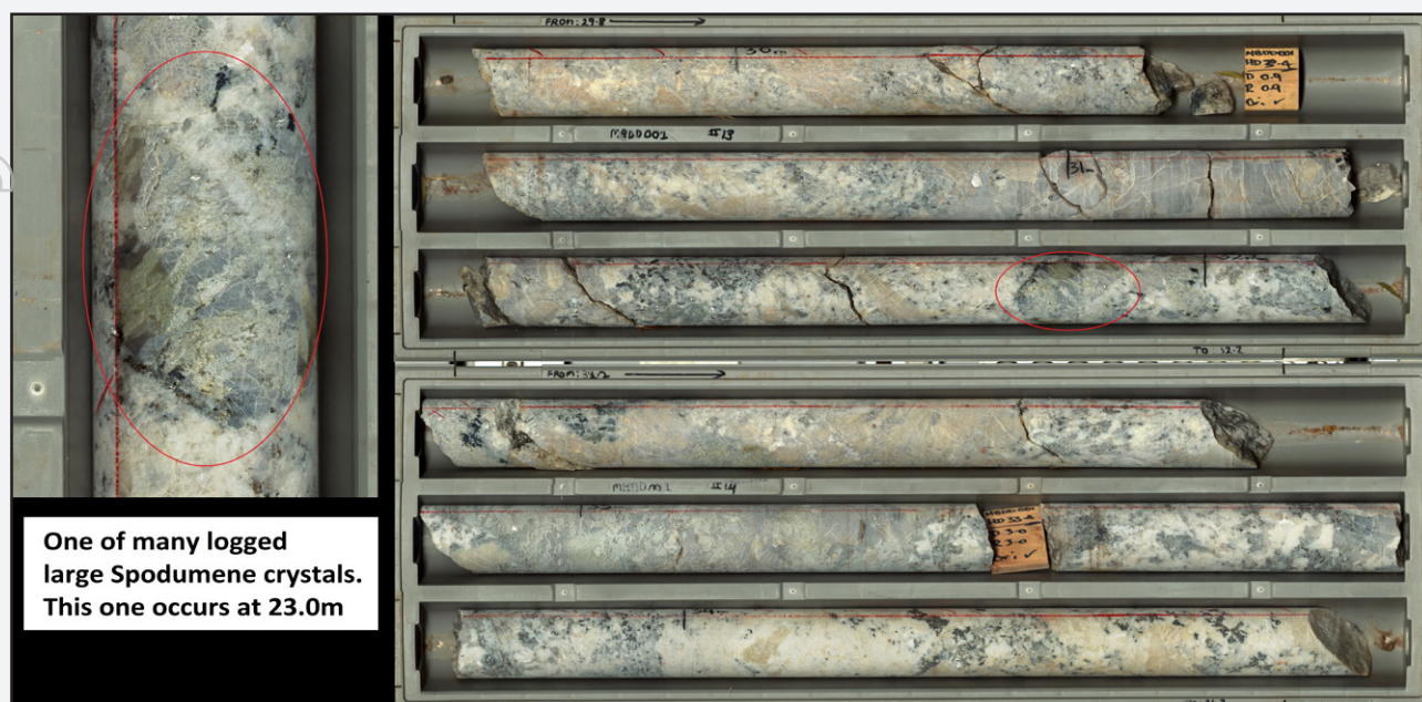
Figure 9. Core photos of pegmatite intervals from MBDD0001 showing spodumene mineralisation (LHS) at 32.0m and spodumene in pegmatite between 29.8-34.9m (full intersection of 29.8-45.8m not shown)
