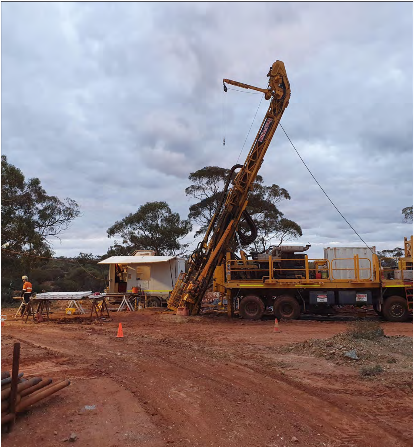
Figure 2: PQ metallurgical drilling underway at Mt Mulgine
