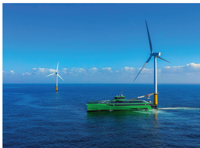
Figures 1 & 2: The Damen FCS 7011 vessel "Aqua Helix", featuring the VEEM Marine VG520SD gyrostabilizer, won the Offshore Energy Vessel of the Year award in June 2022. This revolutionary "walk to work" vessel is capable of continuously sailing at speeds of up to 40 knots to enable short transit times.
