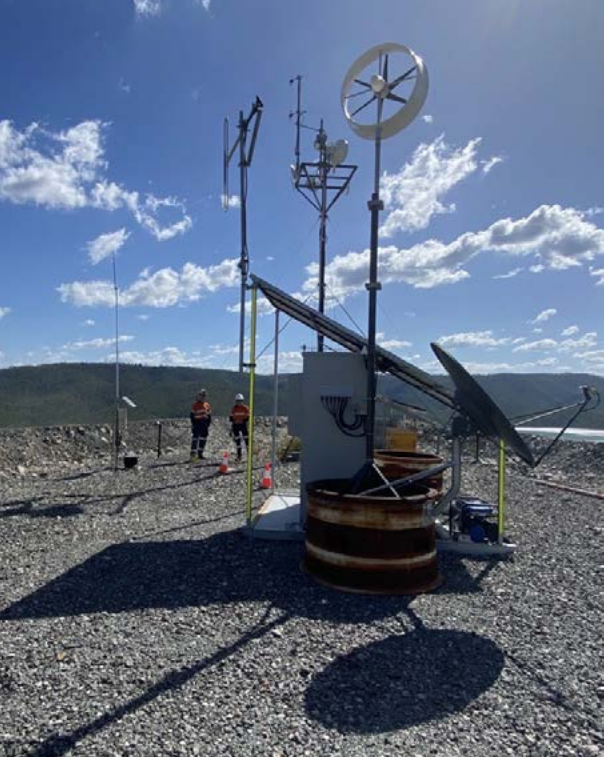
Solar and wind powered weather station at Mt Rawdon
