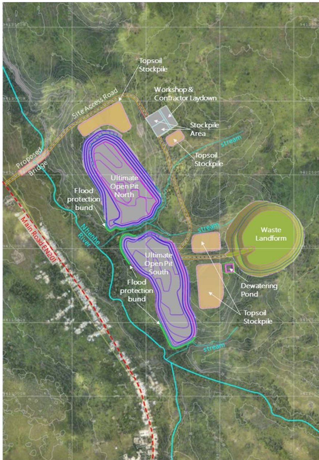
Figure 10-3 Căcata Phosphate Mine – Overall Site Layout
