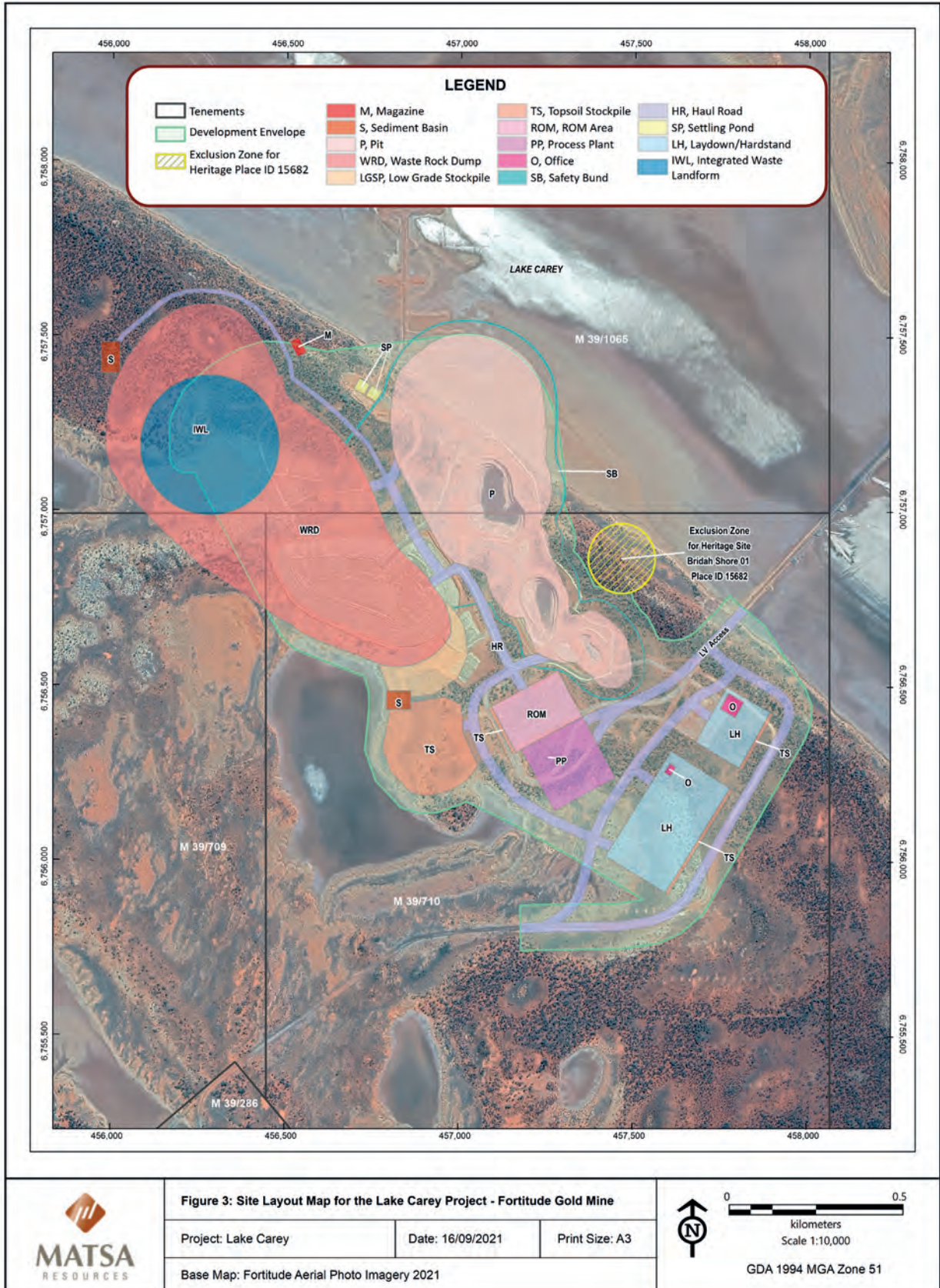
FIGURE 10: Proposed mine layout for Fortitude Gold Mine including potential mill and tailings facilities
