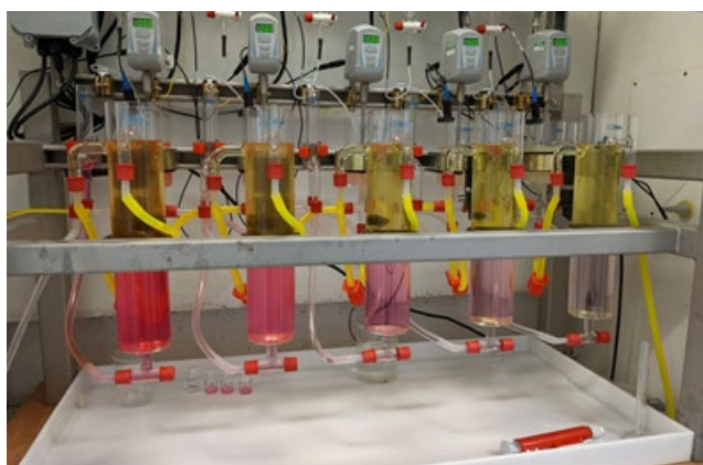
Figure 10: Mixer Settler pilot plant located at Queens University Ionic Liquids Laboratory (QUILL) at QUB.
