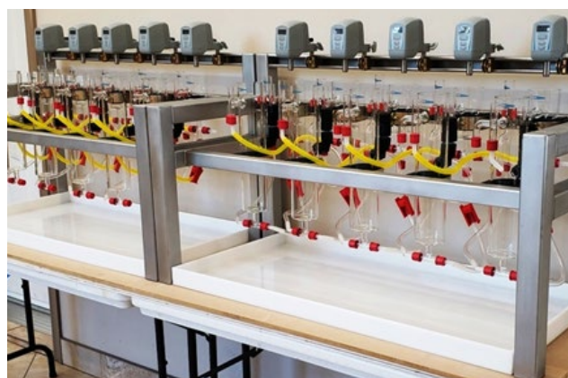
Figure 10: Mixer Settler pilot plant located at Queens University Ionic Liquids Laboratory (QUILL) at QUB.
