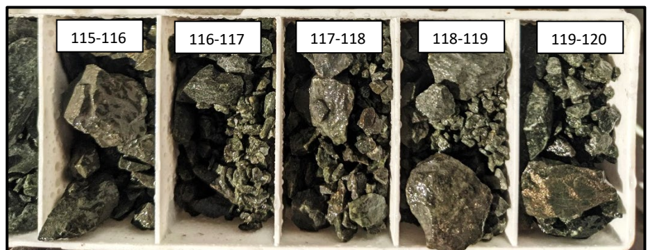
Figure 1 — RC chips with disseminated sulphides (5%) in NRC346
