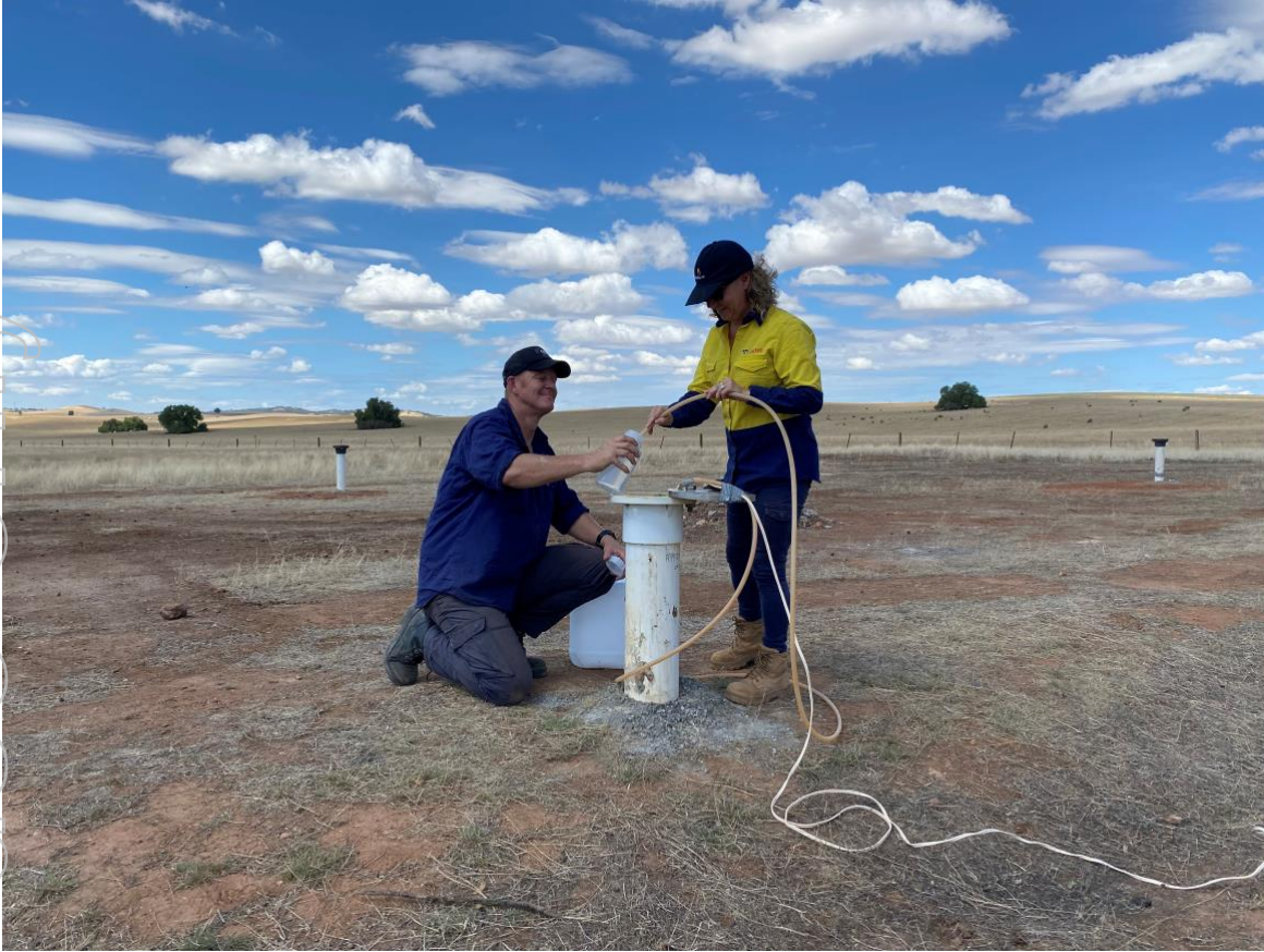
Photo 4: Push-Pull Tracer Trials Underway at Kapunda
