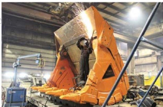
Repair of buckets at CTS in Ngezi
