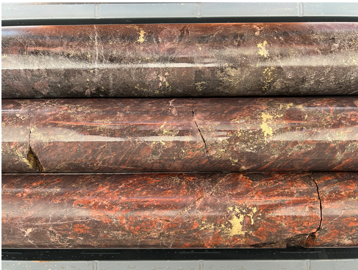
Figure 6: Examples of heavily altered volcanics with copper sulphide mineralisation from drill hole WL22DD001 between 575-577.7m. Copper sulphide (chalcopyrite) is yellow
