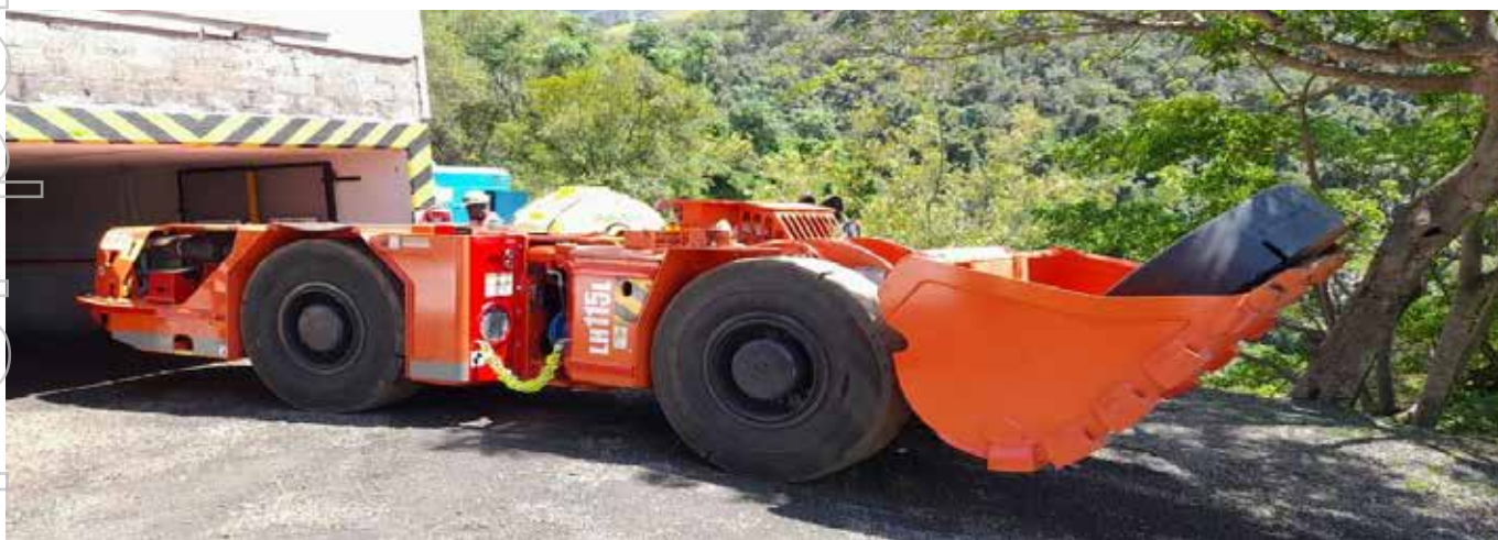
Figure 2: Low-Profile Loader entering Frankfort mine
