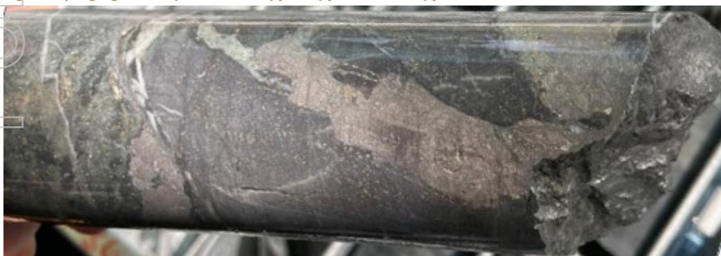
Figure 8 | High grade sulphide (arsenopyrite, pyrrhotite and pyrite) mineralisation from RCDD22OKV444, 6m @ 14.10g/t from 323m
