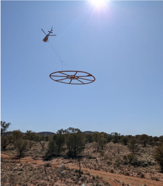
Figure 6. NRG's Airbus AS350B3 Squirrel Helicopter with Towed EM Array
