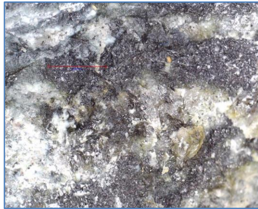
Figure 11: Quartz-biotite altered mafic in 22WAC0030, 49-50m (red bar 5mm)
