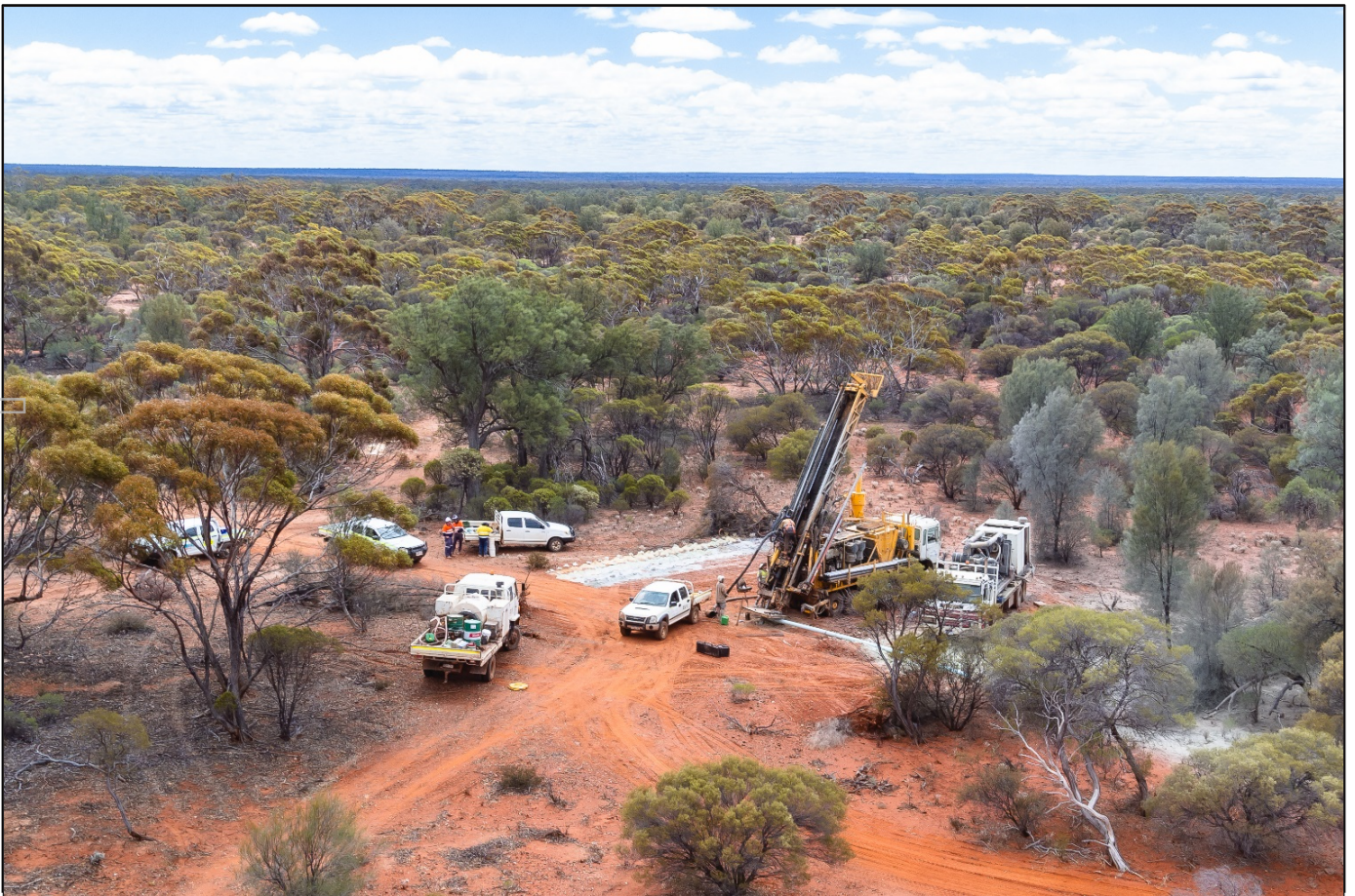
Figure 5; RC drilling in the December Quarter FY22 at the First Hit Project.
