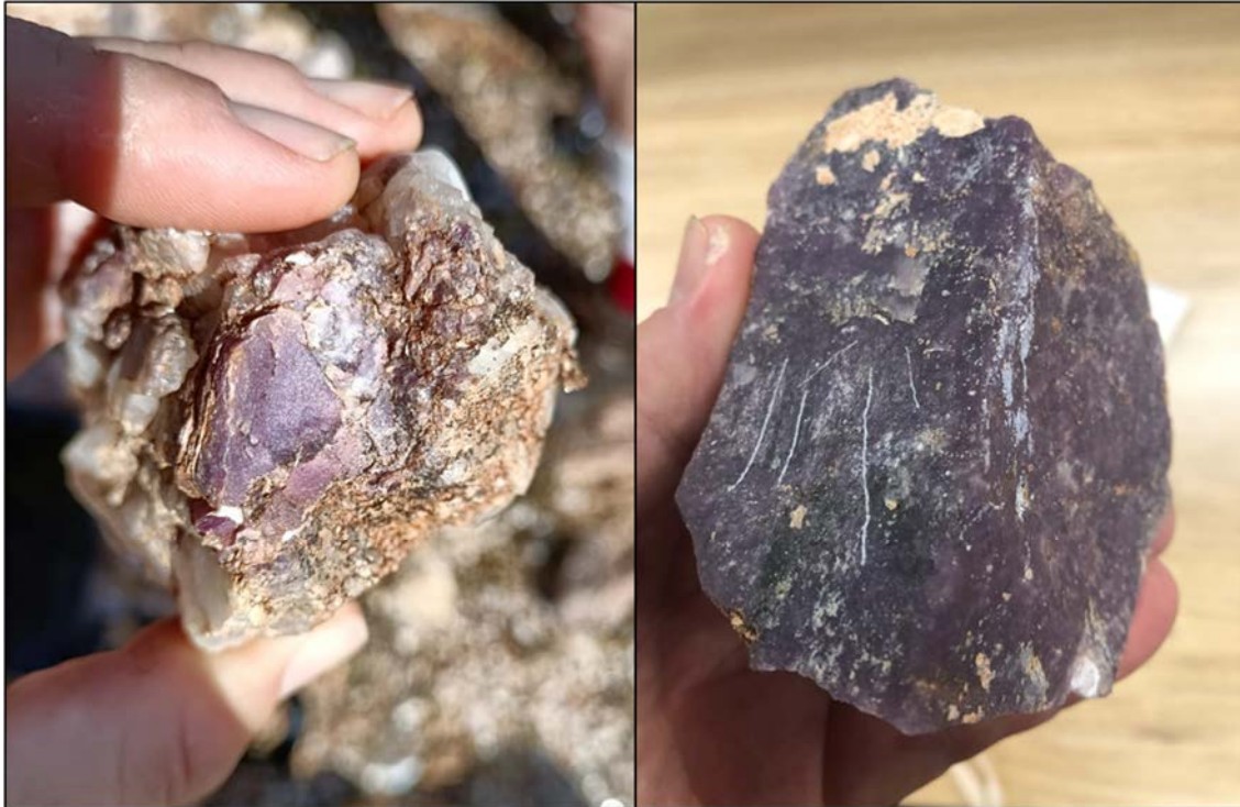
Figure 4 – photos of pegmatites from E29/962 (100% St George) with coarse grained purple crystals that may be indicative of spodumene and lepidolite, subject to confirmation by portable XRD spectrometer and laboratory analysis.
