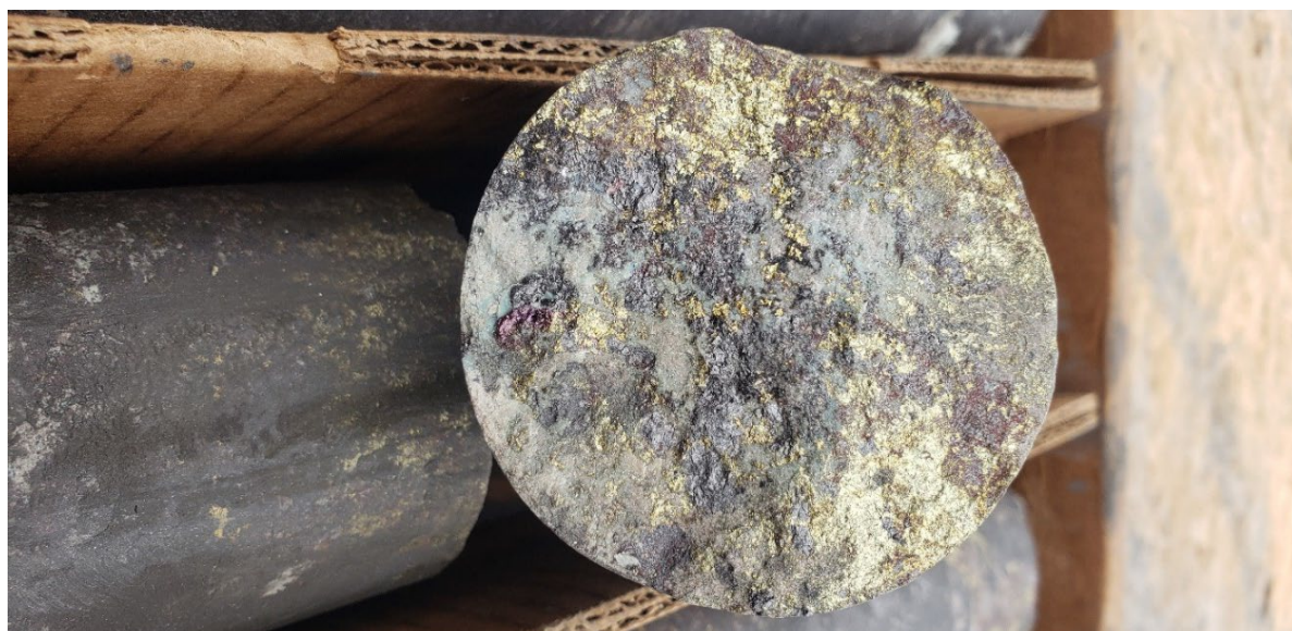
Figure 11: Photo of chalcopyrite and bornite (copper sulphide) within magnetite skarn from approximately 363.91m (1194ft) downhole in drill hole WD22-05.
