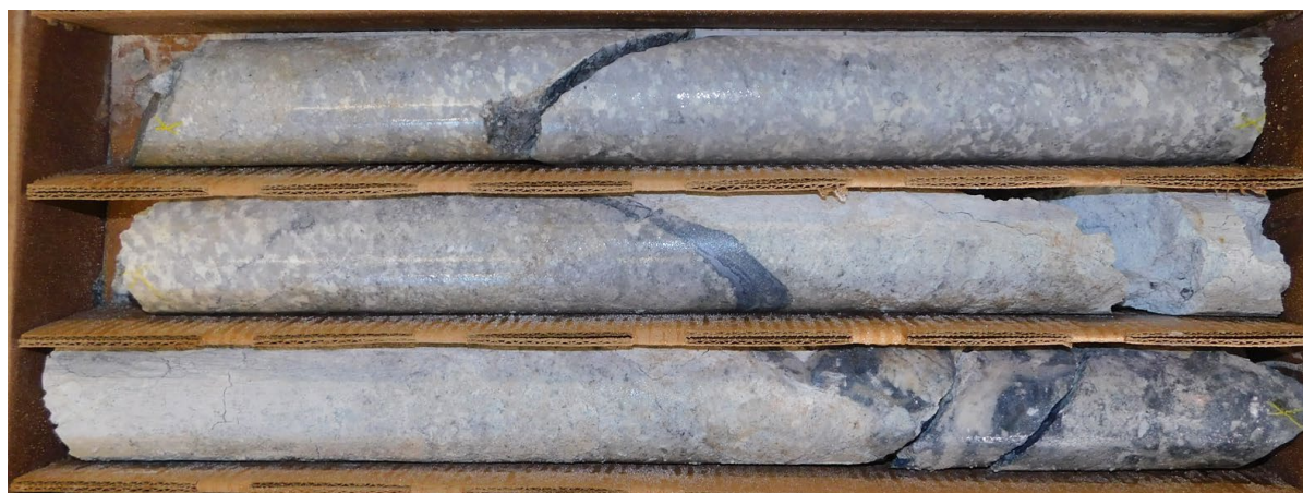
Figure 6: Strong molybdenite veining in drill core from WD22-01 (761 – 763.5m downhole)
