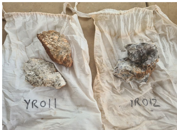
Figure 6. Muscovite and Grey Lepidolite up to 15% by volume in Pegmatite Samples
